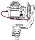
There are four camera control cables: Type-C to Multi USB/Type-C to Type-C USB / Type-C to Micro USB / Type-C to Mini USB. Choose the correct cable corresponding to the USB port type of the camera. For the compatibility details, please visit the official website of ZHIYUN (www.zhiyun-tech.com) and check the CRANE 4 Camera Compatibility List.
