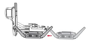
In order to have the best image transmission, please rotate the antenna to the position as shown in the image. The antenna can only be rotated in one direction. Please rotate properly. For more details, please read the user guide of transmitter Al.
