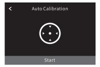
When performing auto-calibration, please make sure that the gimbal is balanced, the three axes are unlocked and the gimbal is straightly put on a flat surface. Please don't touch the gimbal when calibrating.
